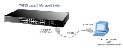
A terminal program is required to make the software connection to the WGS3 Layer 3 Switch. Windows' **Hyper Terminal** program may be a good choice. The Hyper Terminal can be accessed from the **Start** menu.
